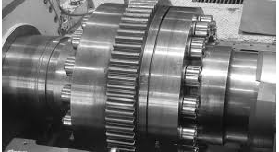
Superbolt replacements for 12 fitted studs on a 400-MW steam turbine: 12 EzFit mechanical expansion bolts, each secured by two multi-jackbolt tensioners. Torque required was only 55 ft-lb
