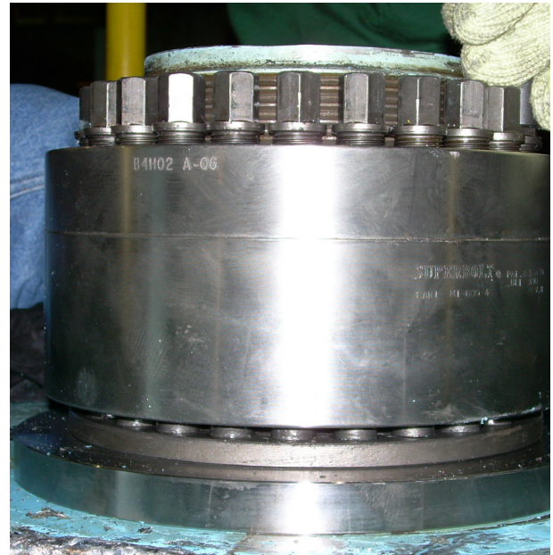
6" diameter Superbolt MT tensioner, with optional ring.
