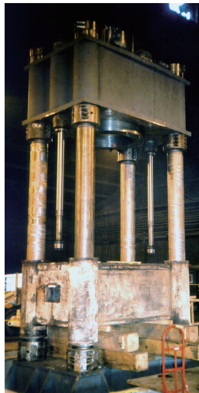
Forging press columns tensioned by 16-1/2" Superbolt split nuts.
