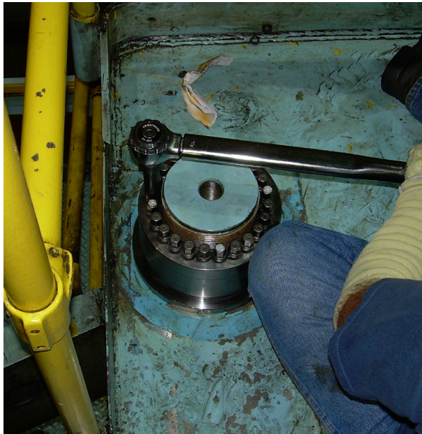
6" Tie Rod Nuts. Jackbolt torque is only 163 lb•ft (220 Nm), making installation and removal safe and easy!
