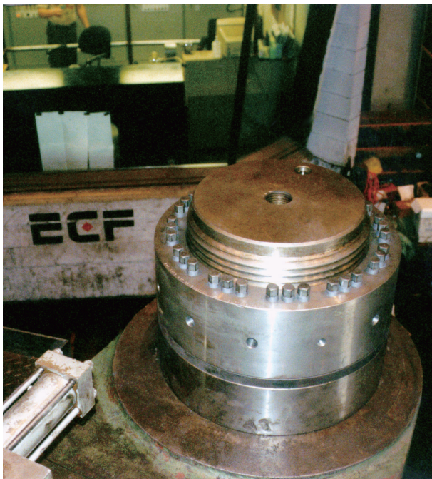
Superbolt nut style tensioners on 400 mm (approx. 15.75") columns for a 1,500 ton underground hydraulic forging press.
