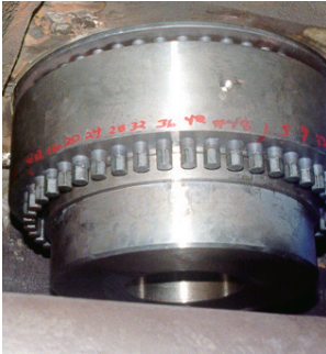
18" Superbolt tensioner creates 2,625,000 lbs (11,700 kN) of preload with only 275 lb•ft (370 Nm) of torque.
